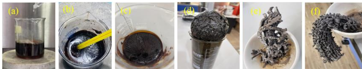
Figure (1): Photograph of (a) nitrates-citrate solution, (b) The solution after the Adding of ammonia, (c) dry gel, (d) Dry bulk temperature of 150°C, (e) Dry bulk temperature of 250°C and (f) auto combustion and become Nano powder ferrite.
