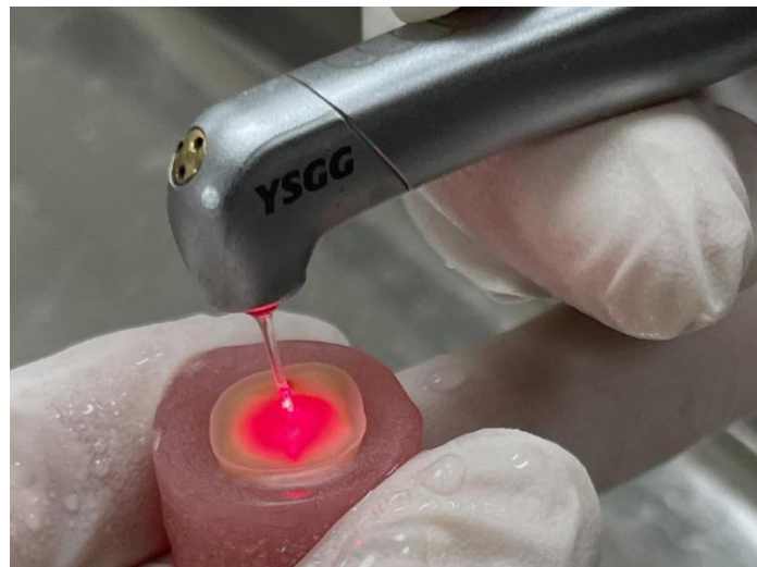
Figure (2): Surface treatment using Er,Cr:YSGG laser beam.
