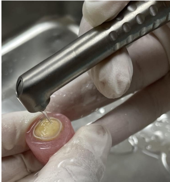
Figure (1): Surface treatment using ER: YAG laser beam.
